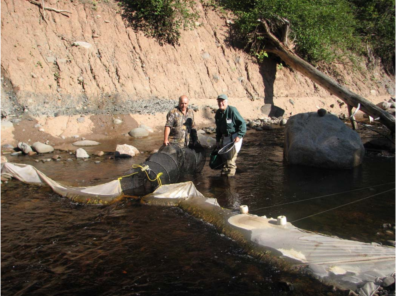
Figure 10. Fyke net in place 400 meters from the Annapolis Basin positioned to capture fish moving upstream. Roy Bertaux (left) and Reg Baird (right) were the local experts conducting the survey. Image by Barb Baird.
