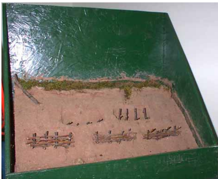
Model Showing Construction of Live Sills
