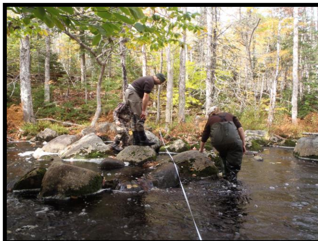
Figure 47. Field crew estimating substrate composition and instream cover along a transect.
