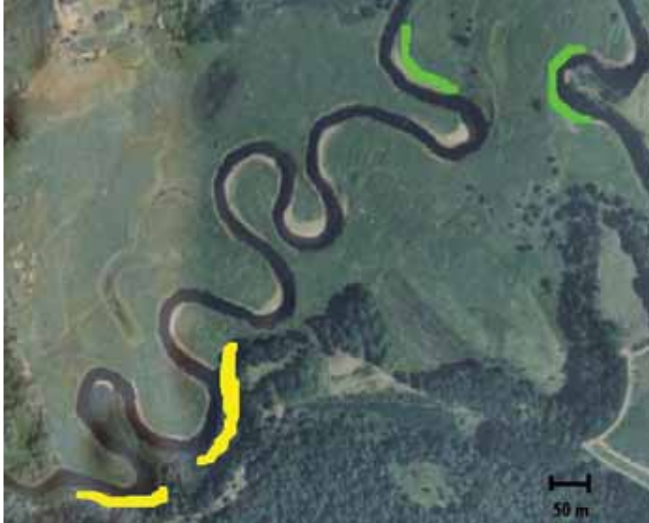
Figure 16- Aerial photograph of The Town of Middleton property. The yellow line represents the location of the container stock spruce trees, the green line represents the location of the live willow stakes.
