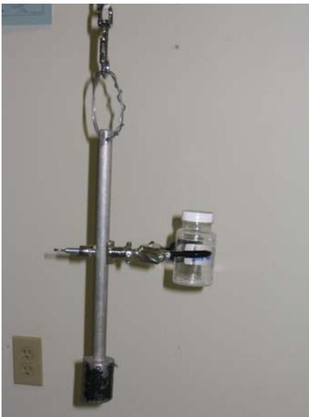
Figure A1 — Collection Unit Used for Fecal Coliform Samples in 2004.
