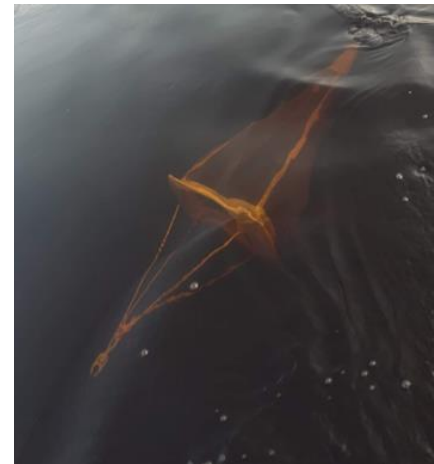
Figure 16. Stationary plankton net deployed in the Annapolis River to collect striped bass eggs.
