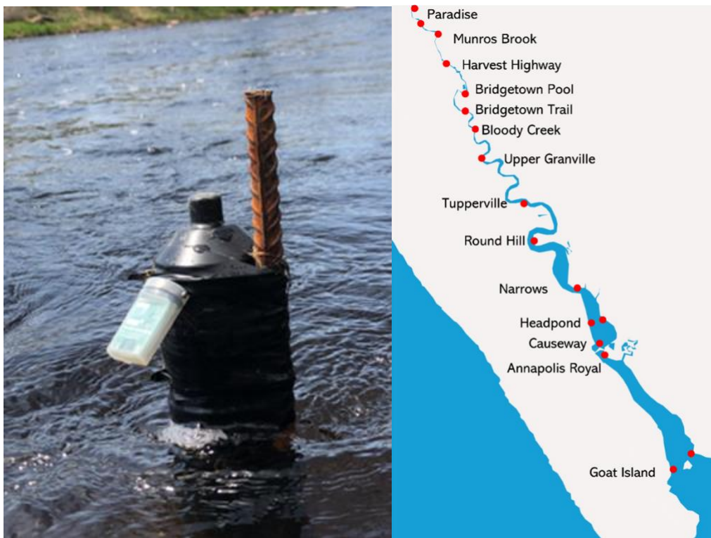
Figure 6. Left: VEMCO VR2W receiver with Onset HOBO temperature logger affixed to rebar in the Annapolis River (Actual receiver submerged, exposed for visual representation). Right: 18 site receiver array in the Annapolis River, stretching from the Paradise, 10 km above the salt wedge, to Goat Island in the Annapolis Basin.
