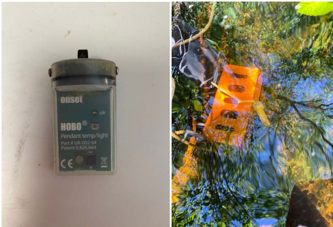
Figure 1. (Left) HOB0 pendant temperature logger. (Right) Temperature logger deployed in the Fales River.
