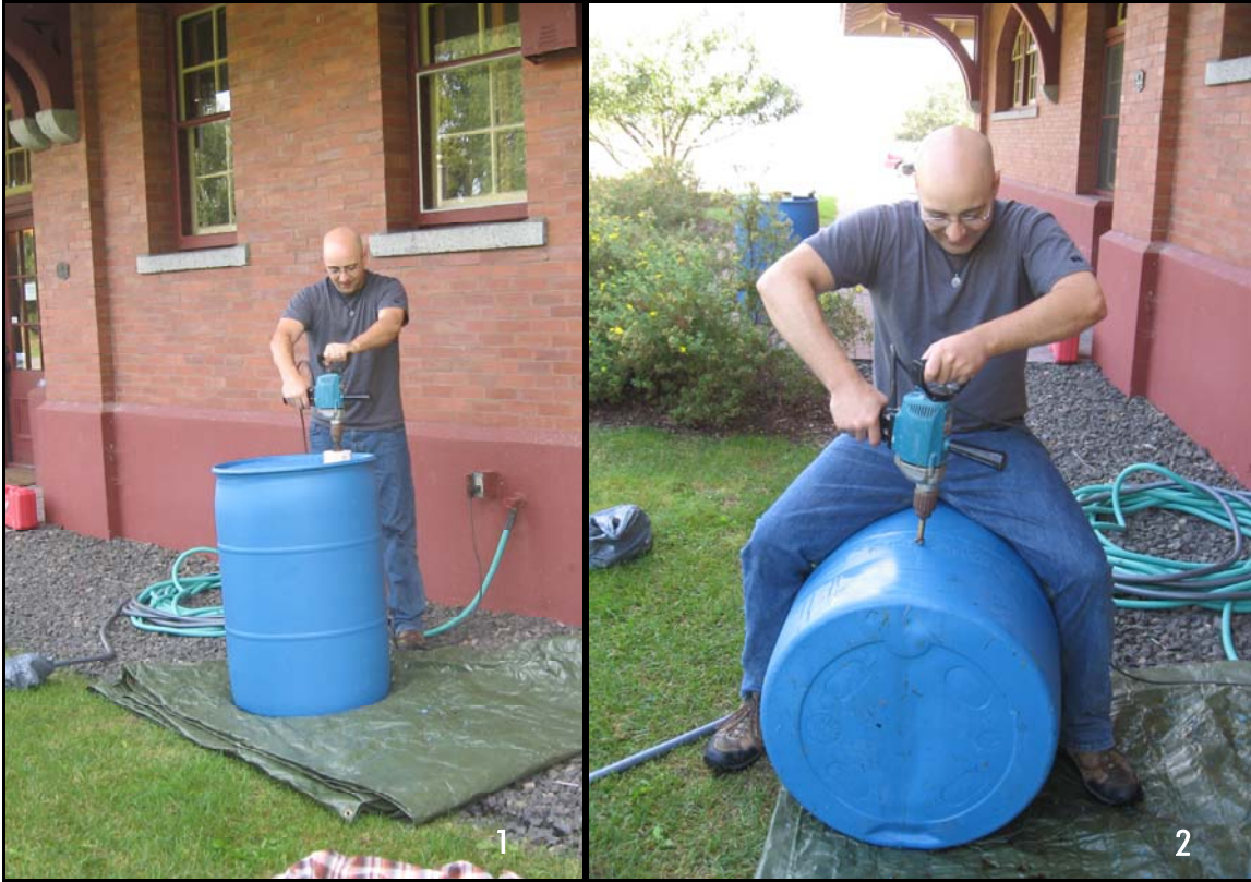
Figure B1. Drilling the hole for the PVC reducer.
