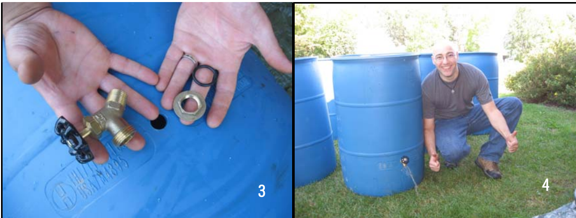
Figure B3. The spigot, o-ring, and faucet lock nut for the rain barrel.
