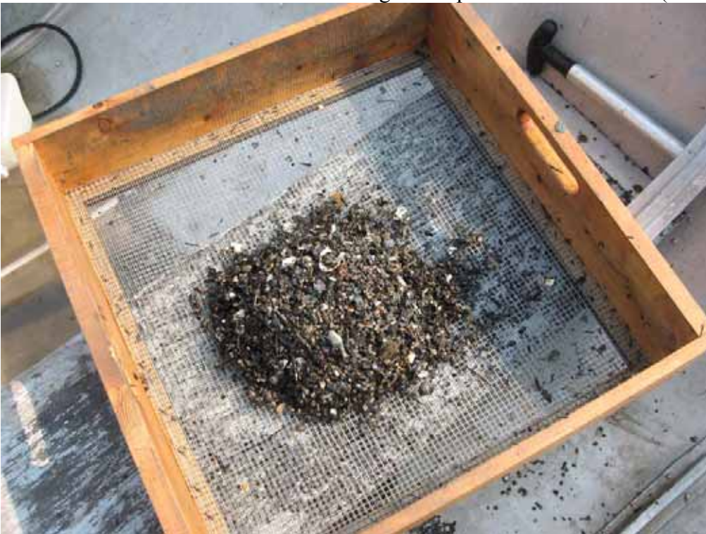
Photo 4: Retained sediment from mesh bag is dumped into screened box (5 mm mesh).
