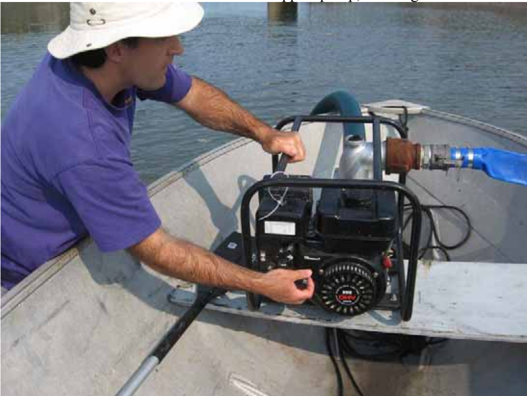
Photo 2: Boat is used in shallow water to support pump, showing intake and exit hoses
