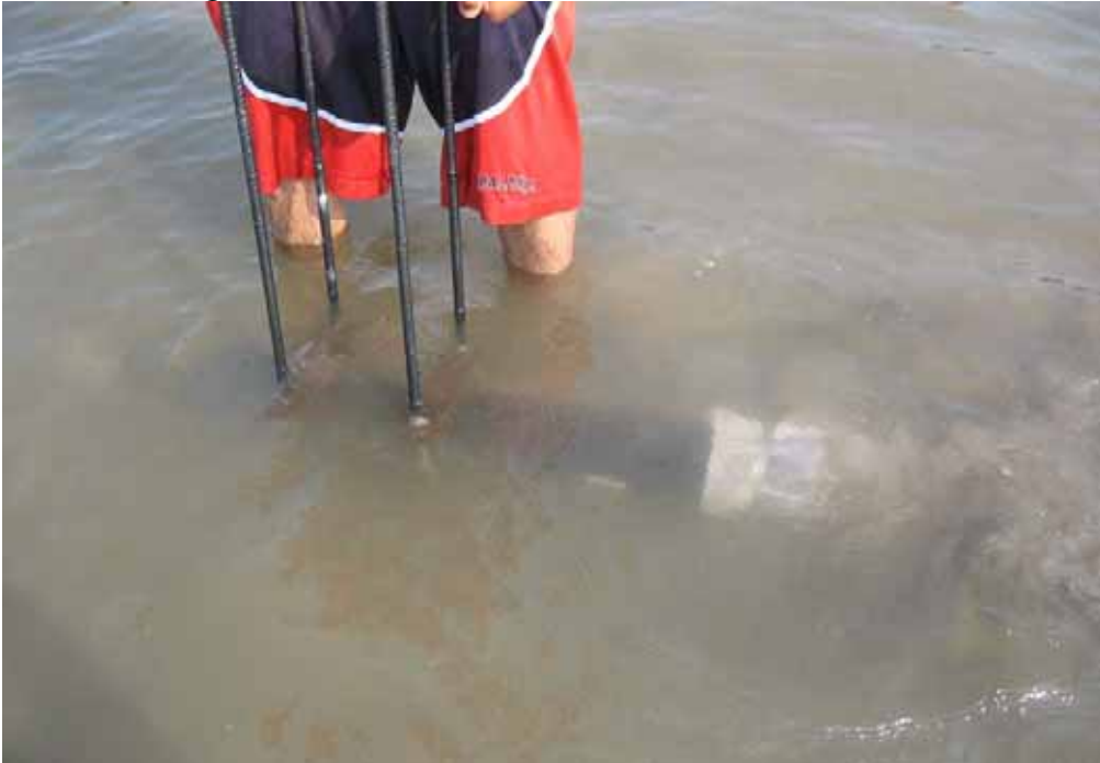
Photo 3: Suction unit being used in shallow water. Note sediment billowing out through white mesh bag.
