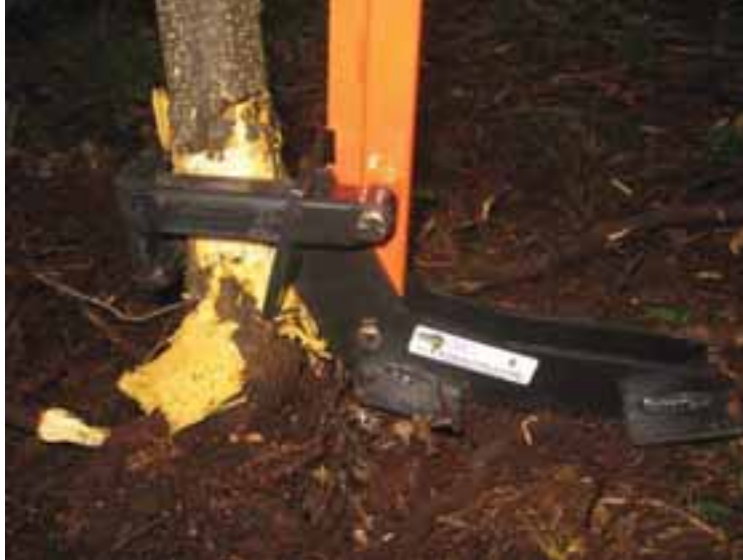
Figure 3- Weed Wrench (Extractigator™) removing a glossy buckthorn stem that was too large to pull by hand.
