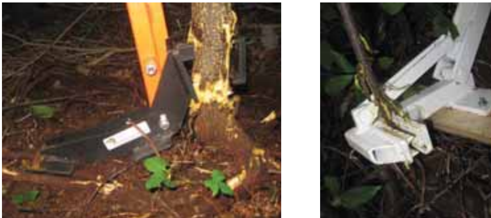
Figure 2- The Extractigator™ weed-wrench (left), and the Puller-Bear™ weed-wrench (right).
