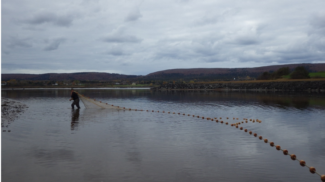
Figure 3. Conducting beach seines in the Annapolis River by walking the seine net out parallel to shore. The 'purse' is identified by the cluster of floats in the middle of the float line.
