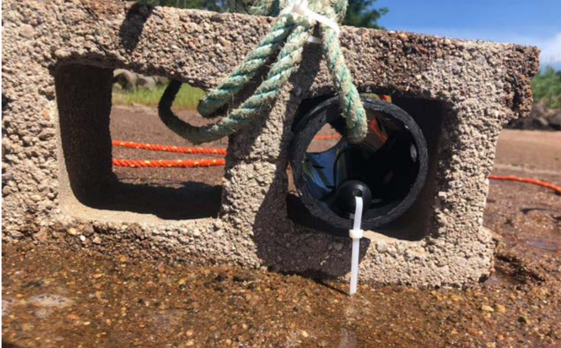
Figure 4. Pressure sensor setup consisting of a single HOBOT water level logger secured inside a PVC tube and anchored by a concrete block.
