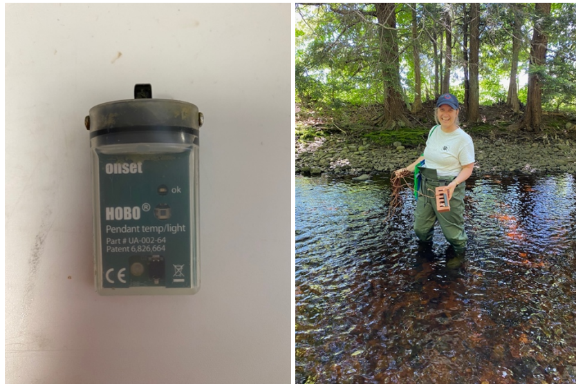
Figure 2. (Left) HOBO pendant temperature logger. (Right) CARP staff, Brittini Scott, deploying a temperature logger.
