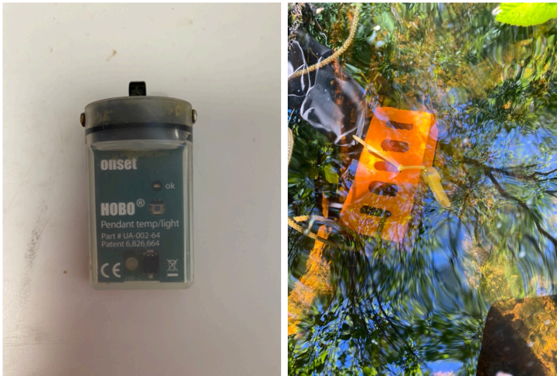
Figure 6. (Left) HOBO pendant temperature logger. (Right) Temperature logger deployed in the Fales River.
